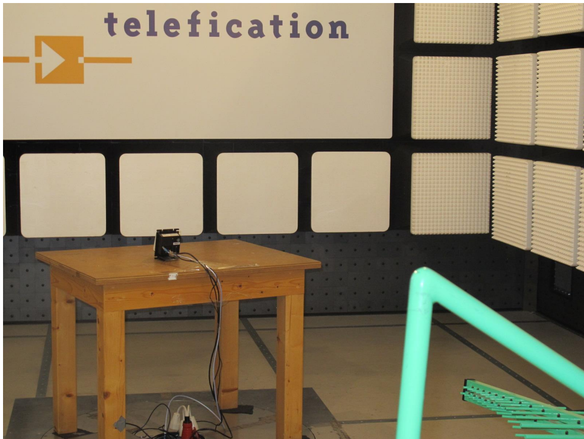
Photograph 2: Equipment under test in Semi Anechoic Room (SAR) (0.03 – 1 GHz)
