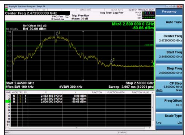
,Plot 2,Band Edge-802.11b,2462MHz
