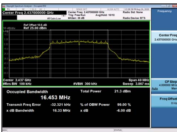
6dB Bandwidth-802.11g,2437MHz
