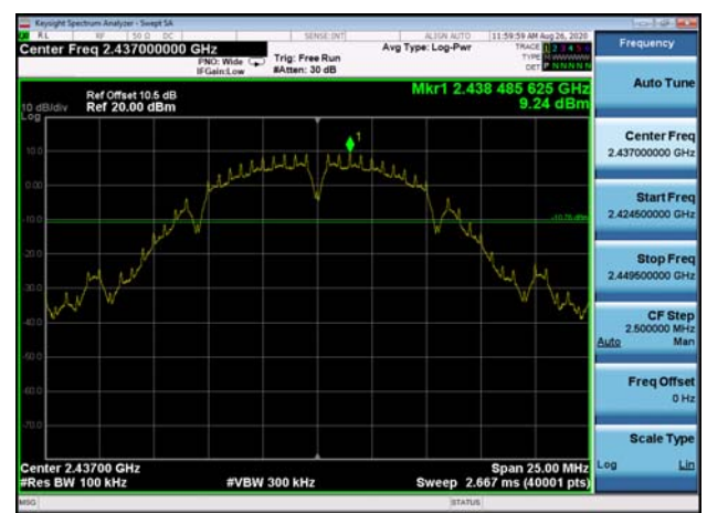
,Plot 2,Band Edge-802.11b,2412MHz
