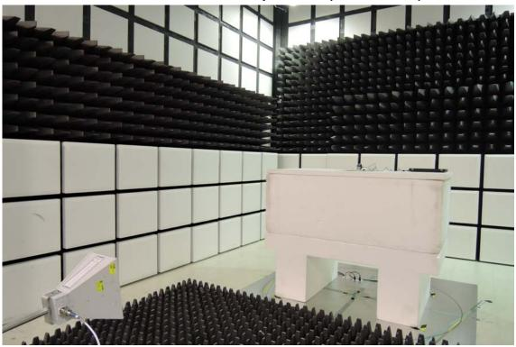
Radiated Emission Set up Photos (Front View)
