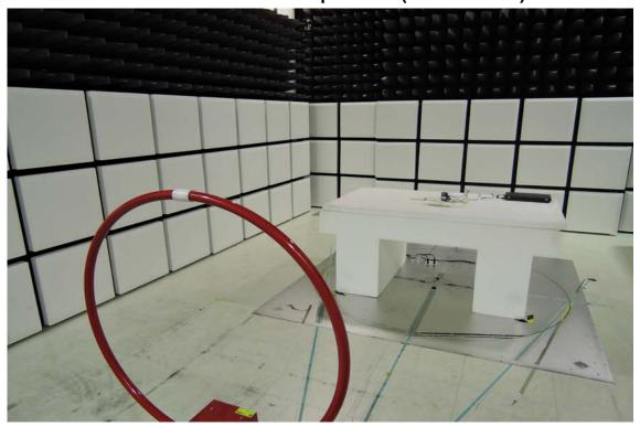
Radiated Emission Set up Photos (Below 1GHz)
