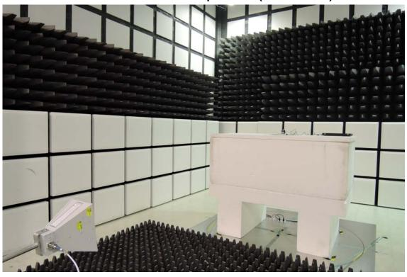
Radiated Emission Set up Photos (Front View)
