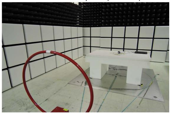
Radiated Emission Set up Photos (Below 1GHz)
