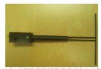
Figure 1 – MVG COMOSAR Validation Dipole
