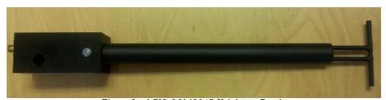
Figure 1 – MVG COMOSAR Validation Dipole
