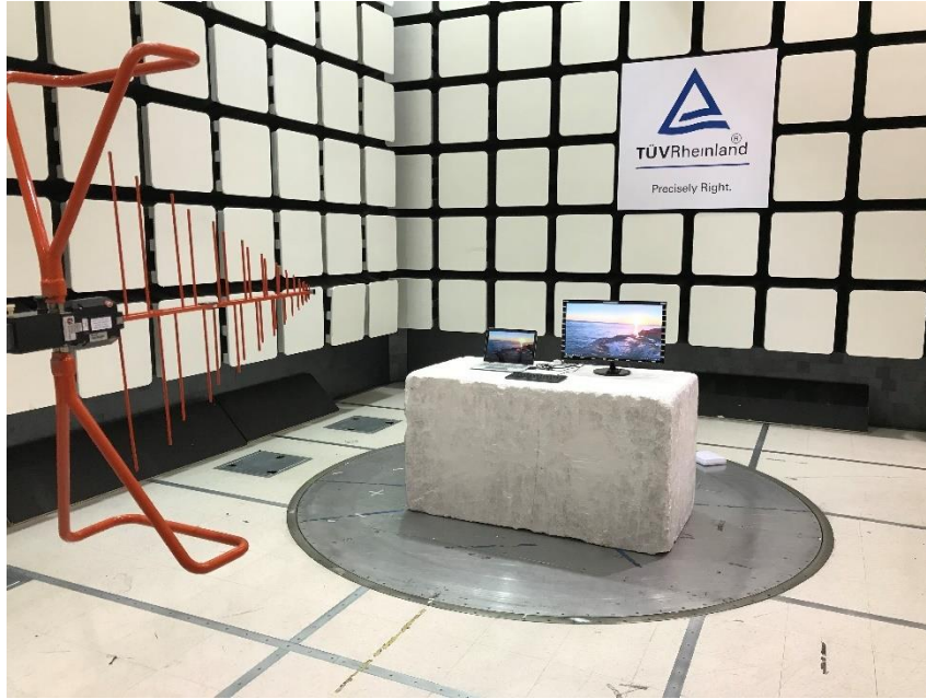
Figure 2: 30 - 1000 MHz Radiated Emissions Test Setup - Front
