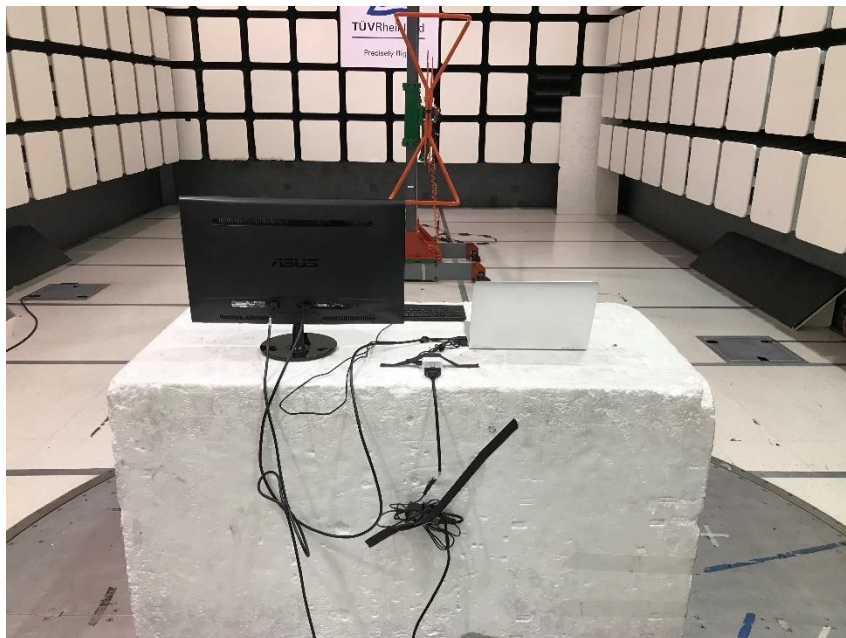
Figure 3: 30 - 1000 MHz Radiated Emissions Test Setup – Back
