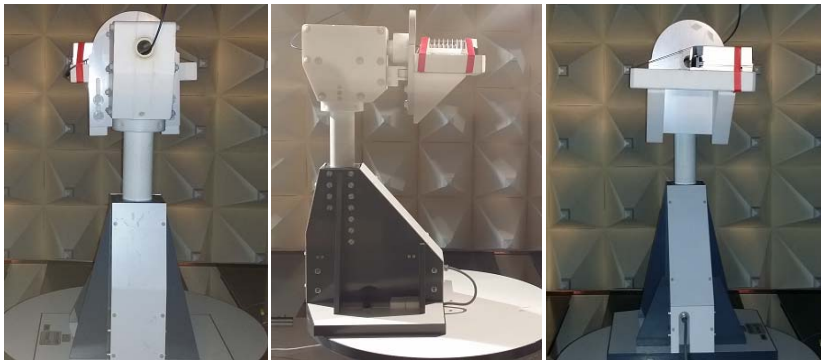
Fixed elevation angle 180°, Azimuth angle is swept from -90° to 90° The pictures show position of DUT for -90°, 0° and 90°
