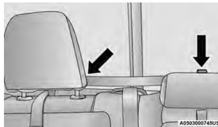
Tether Strap Through Outboard Tether Strap Loop And Attached To Center Tether Strap Loop
