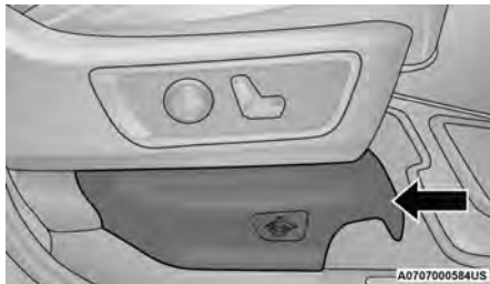
Pull Jack Access Cover From Front
