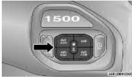
Five-Position/ On-Demand Transfer Case — GT Models
