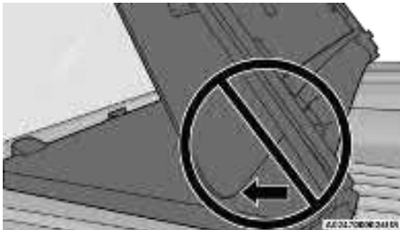
Incorrect Folding – Will Cause Damage
