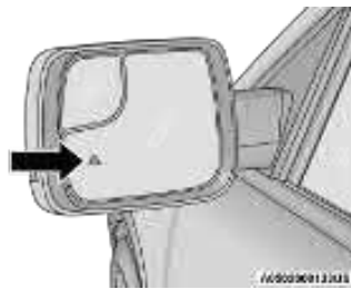
Warning Light Location
