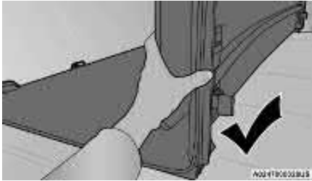
Correct Folding – Hold Panels Together
