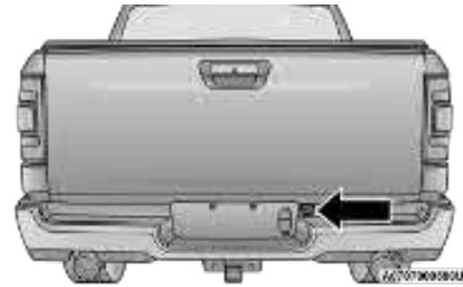
Access Hole Cover Location
