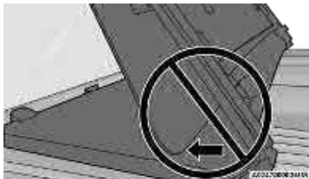
Incorrect Folding – Will Cause Damage
