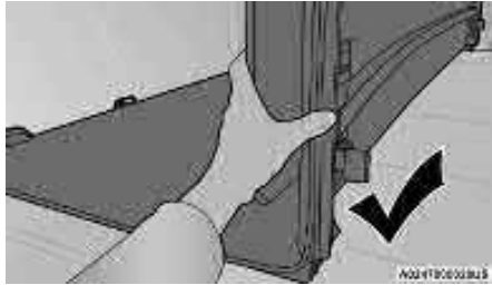
Correct Folding – Hold Panels Together
