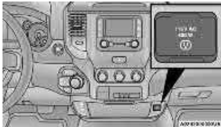
Center Stack Power Inverter
