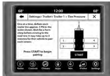
Trailer Tire Pressure Pairing
