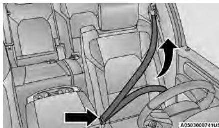
Positioning The Lap Belt
