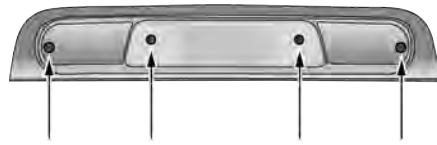
CHMSL Mounting Screw Locations
