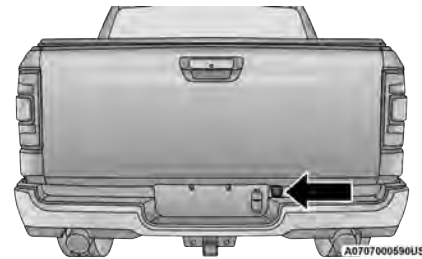
Access Hole Cover Location
