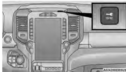
Power Outlet – Top Of Center Stack
