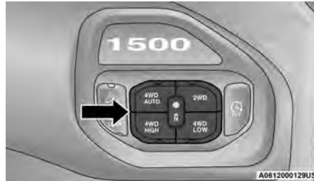
Five-Position/ On-Demand Transfer Case — GT Models
