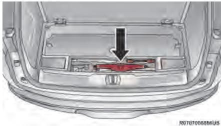
Jack And Tools Storage Location
