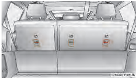
Tether Anchorages (3rd Row Bench)
