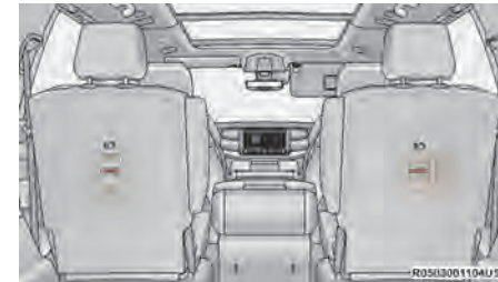
Seven Passenger Top Tether Anchorages (Captain's Chair)
