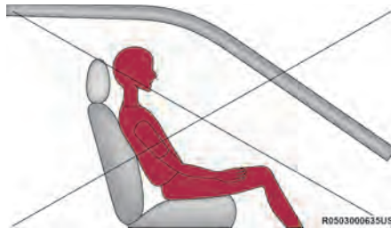
Not Seated Properly
