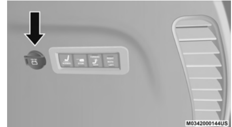
Rear Power Outlet
