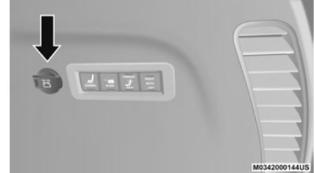
Rear Power Outlet
