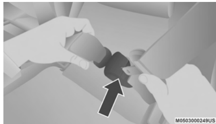
Detaching Mini-Buckle With Seat Belt Tongue
