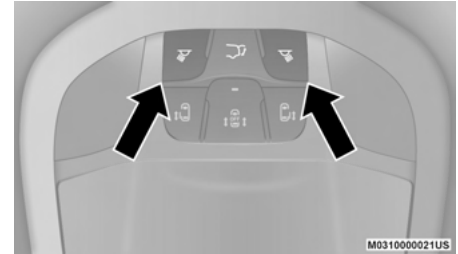
Courtesy Light Switches
