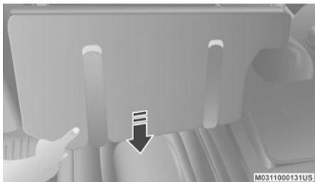
Extend Floor Panel
