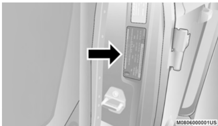
Example Tire Placard Location (B-Pillar)
