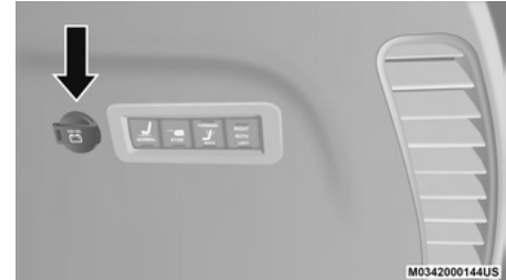
Rear Power Outlet
