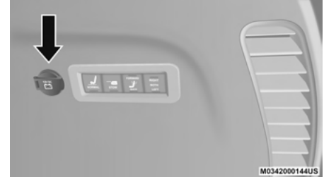
Rear Power Outlet
