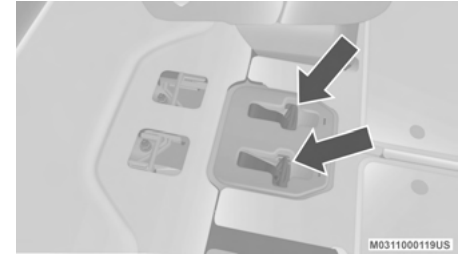
In Floor Detent Guides
