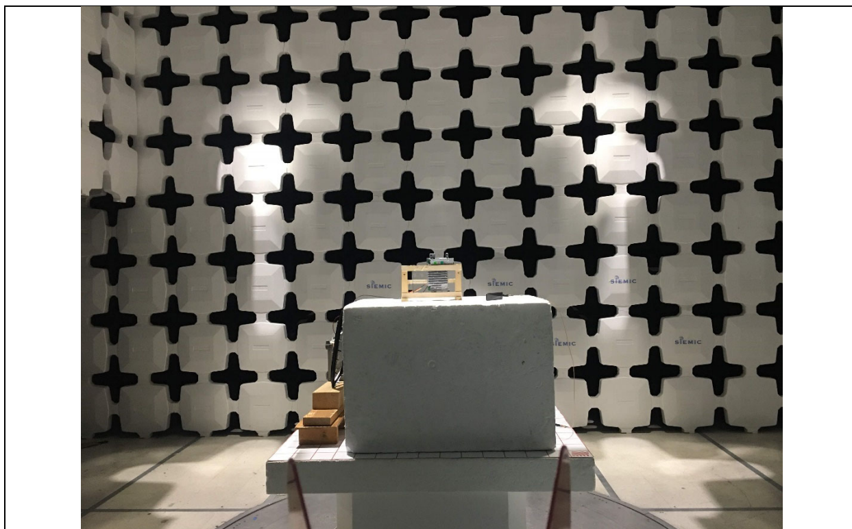
Radiated Emission Test above 1GHz Front View
