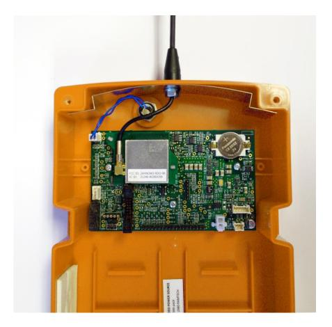
**Board Assembly mounted in horizontal configuration**
