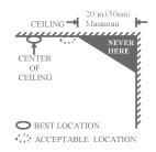
Figure 5: Recommended best and acceptable locations to mount smoke detectors
