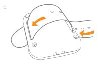
If you want to mount the Panic Button on the wall, you can use the included tape. Put the double adhesive tape on the back of the device and press firmly on the device with the tape to make it stick to the wall.
