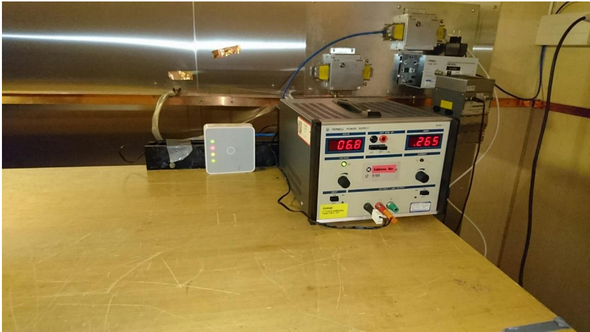
Power line Conducted emission – DC only
