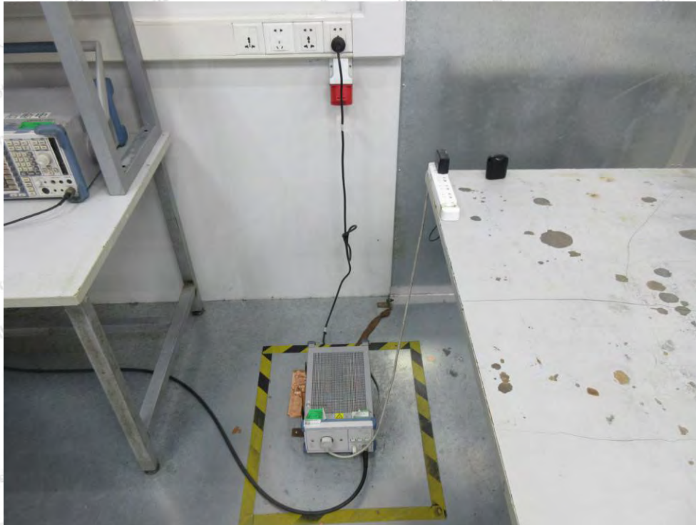
Photo of Power Line Conducted Emission Test
