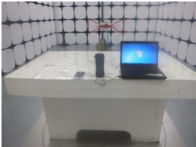
Radiated Spurious Emissions Test Setup Below 1GHz
