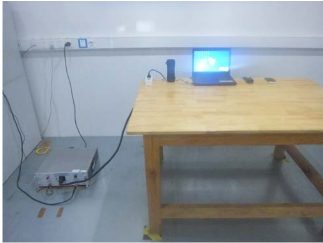
Conducted Emissions Test Setup Front View
