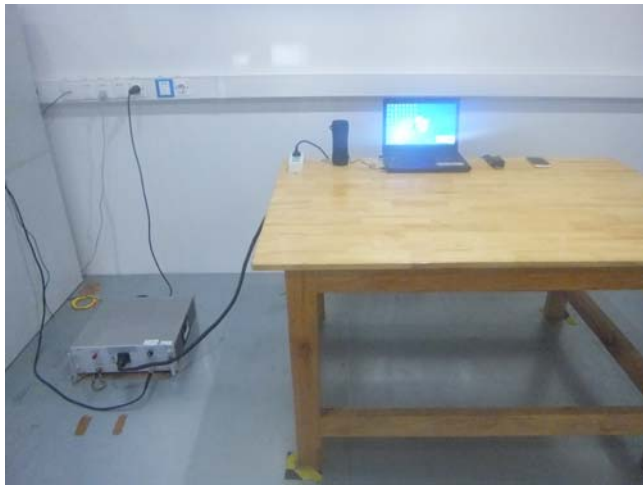
Conducted Emissions Test Setup Front View
