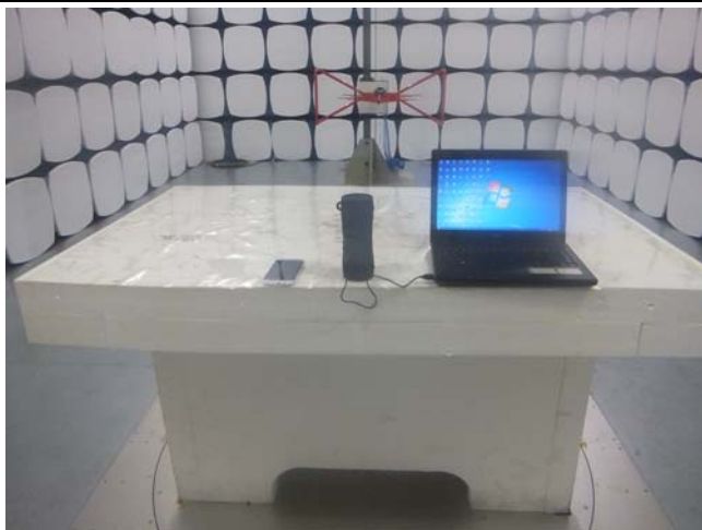
Radiated Spurious Emissions Test Setup Below 1GHz
