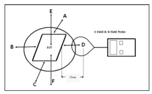
Note: According to KDB 680106 D01 v03r01, section 5(b)(6), 15cm for surrounding, 20 cm for Top test.
