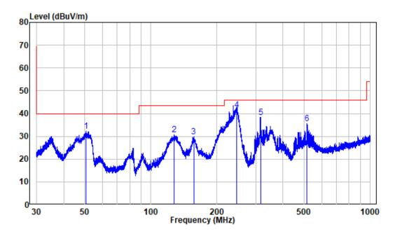
Site : chamber Condition: 3m VERTICAL Job No. : SZNS220602-24345E-RF Test Mode: Full load
