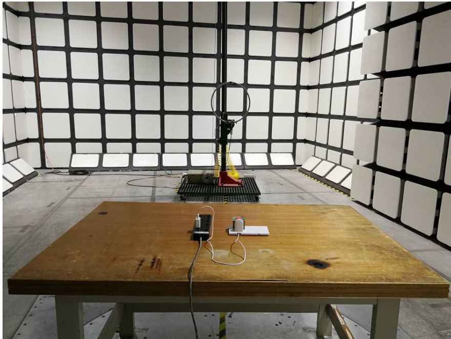
Radiated Emissions View (9 kHz ~ 30 MHz)
