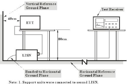
Note: 1. Support units were connected to second LISN. 2. Both of LISNs (AMN) 80 cm from EUT and at the least 80 cm from other units and other metal planes support units.
