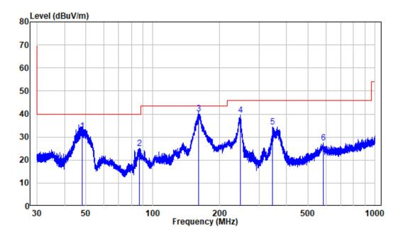
Site : chamber Condition: 3m VERTICAL Job No. : SZNS220602-24347E-RF Test Mode: Full load
