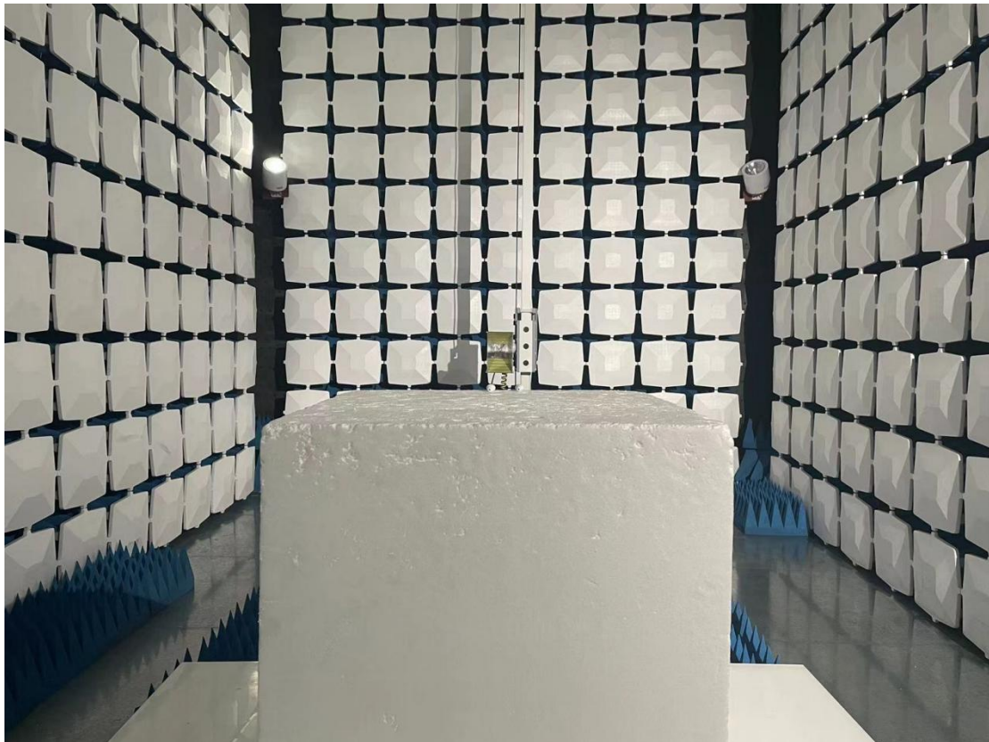
Above 1GHz for radiated emission test setup
