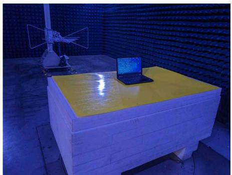
Photo of Radiated Emission Measurement Below 1GHz
