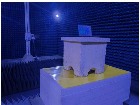
Photo of Radiated Emission Measurement Above 1GHz
