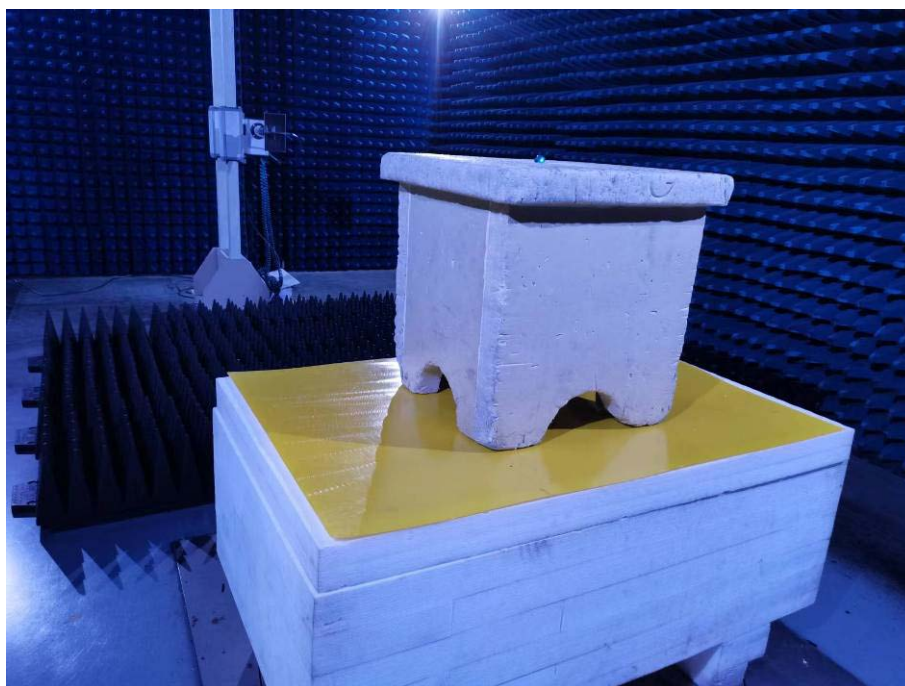
Photo of Radiated Emission Measurement Above 1GHz
