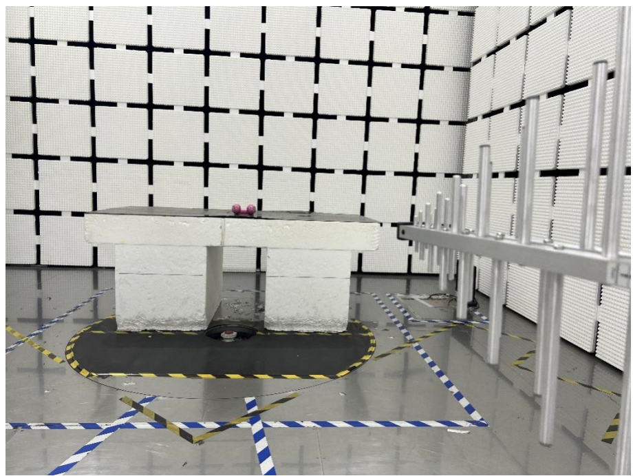
Radiation Emission Test Setup (30MHz to 1GHz)
