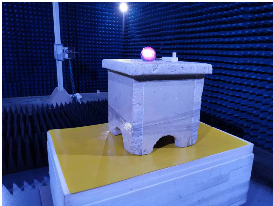
Photo of Radiated Emission Measurement (Above 1G)
