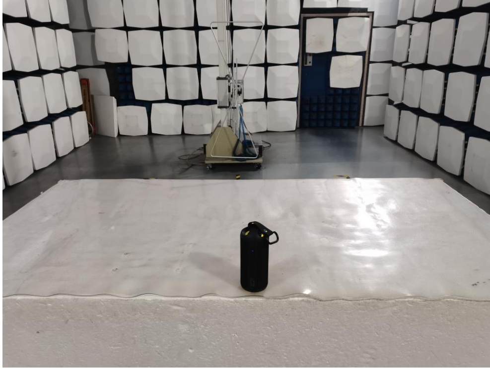
Radiated Emission Test Setup:
