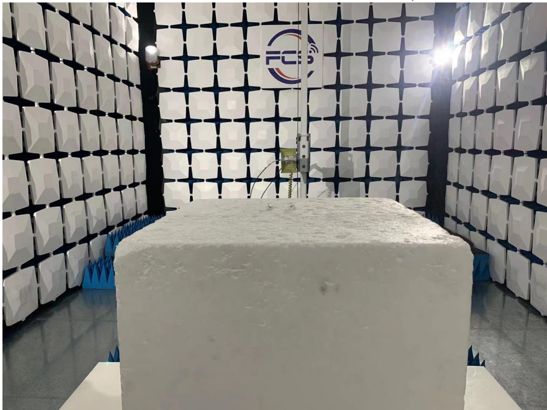
Above 1GHz for radiated emission test setup
