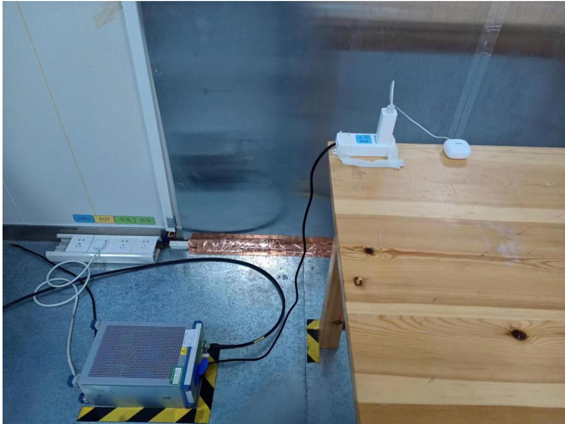
Conducted emission test setup
