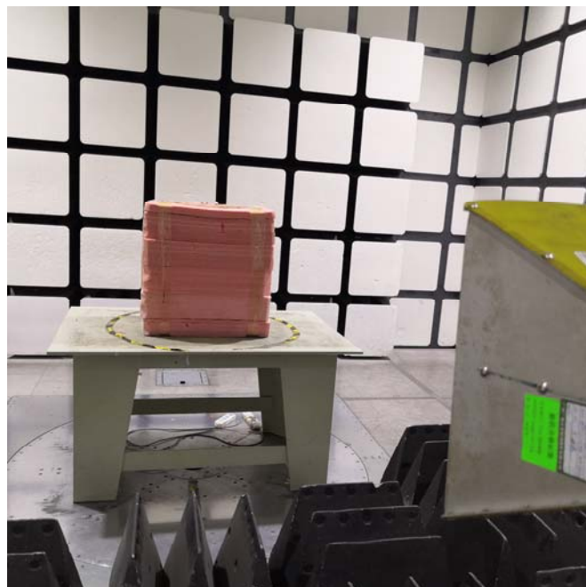
Radiated Emissions View (Above 1 GHz)
