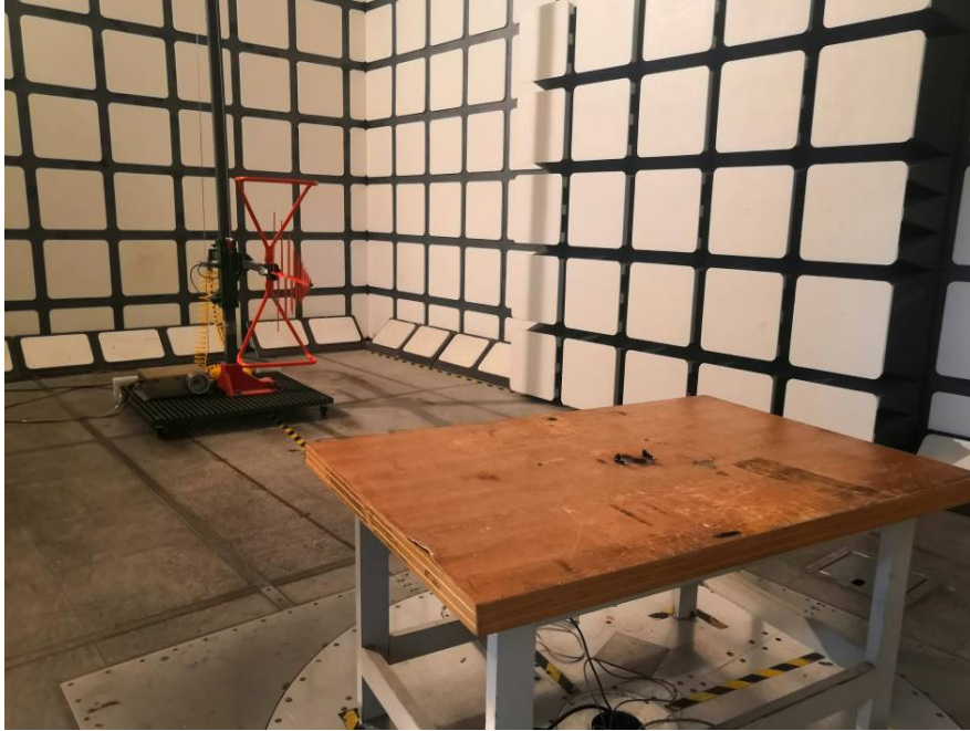
Radiated Emissions View (Below 1 GHz)
