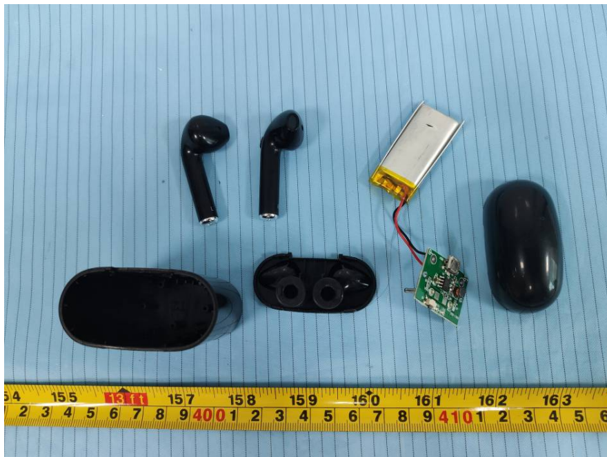
EUT – Charger Cover off View
