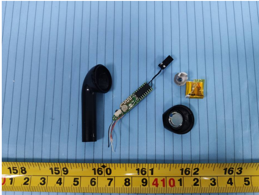
EUT – Earbud Cover off View
