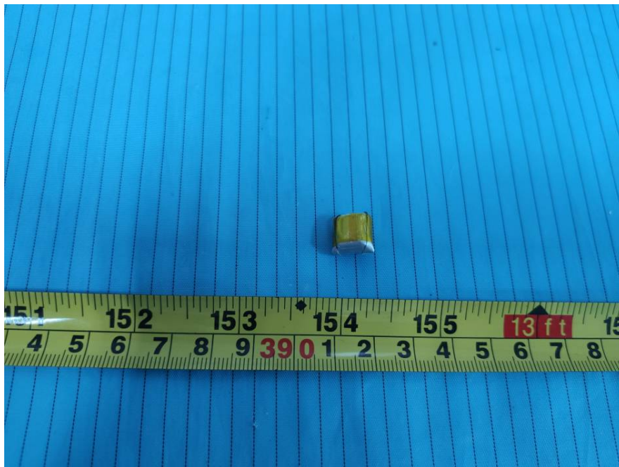
EUT – Earbud Battery Front View
