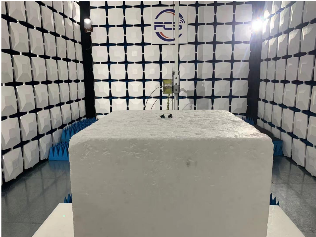
Above 1GHz for radiated emission test setup
