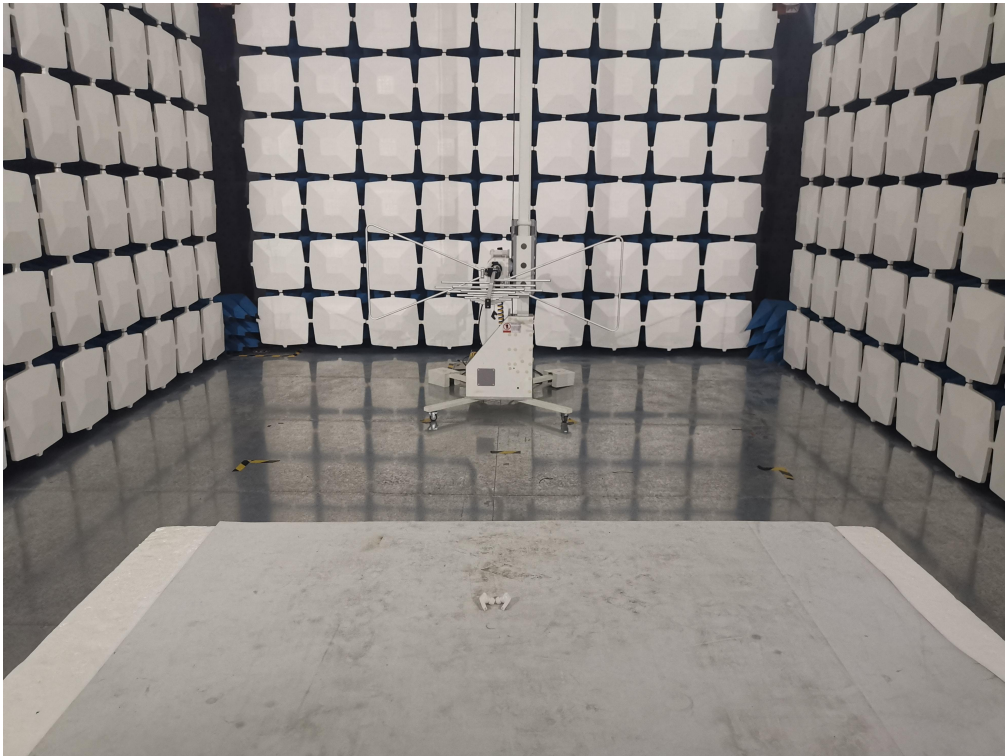
Below 1GHz for radiated emission test setup
