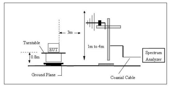
(C) Radiated Emission Test-Up Frequency Above 1GHz
