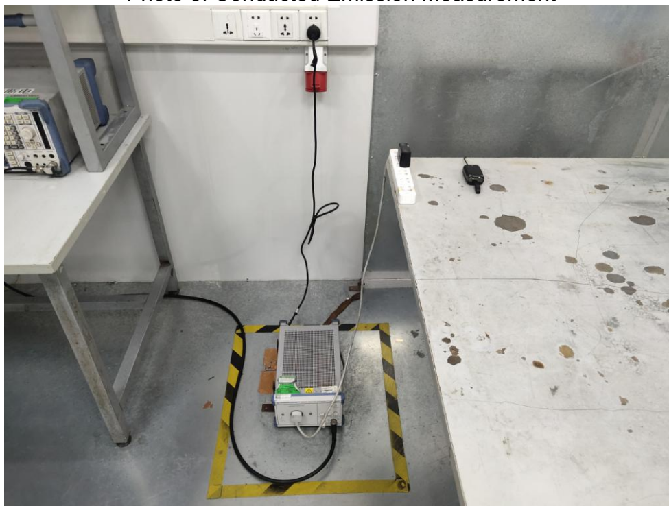
FCC ID: 2AHN6-AUBE210 Photo of Conducted Emission Measurement
