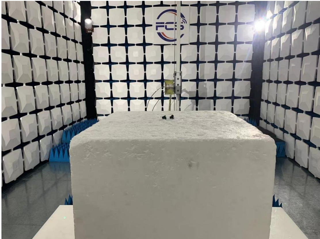
Above 1GHz for radiated emission test setup
