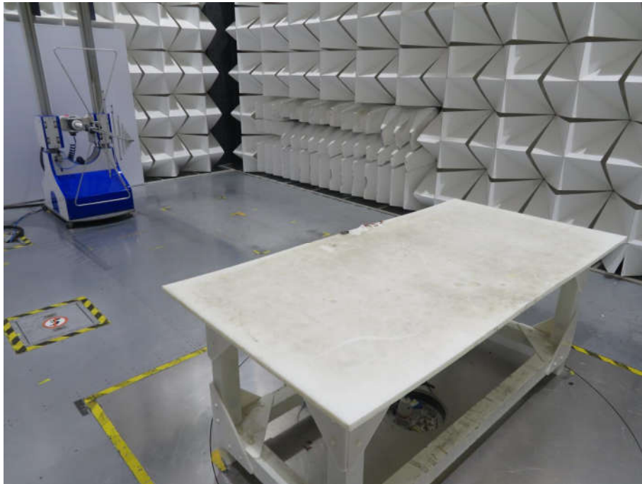
Radiated spurious emission Test Setup-1(30MHz-1GHz)
