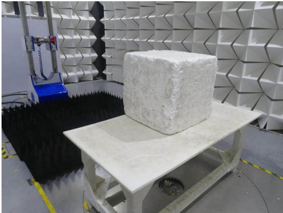
Radiated spurious emission Test Setup-2(Above 1GHz)
